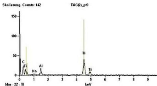
Fig. 2: EDX spectrum of a dark inclusion - detection of aluminum. Ti = Titanium implant.
