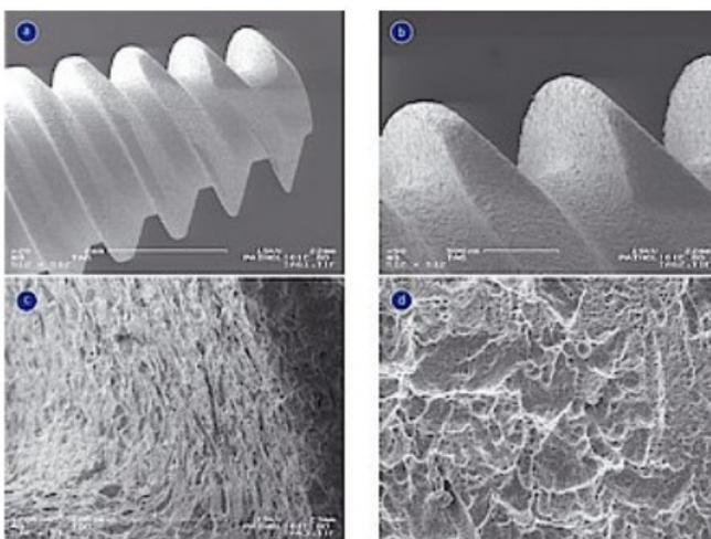
Fig. 1: Scanning electron micrographs of the surface of a sterile TAG implant a) Overview. Clean milled threads. b) Detail shot of the threads. Surface structure of the outer threads, slightly inhomogeneous “frayed”. c) Detail shot of the inner thread. Dark triangular and angular inclusion can be seen. d) Increased surface area. The inhomogeneous structuring of the surface promotes osseointegration.
